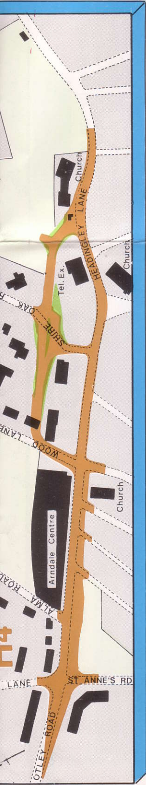
H4 Shaw Lane junction as Scheme H3, plus a one-way system between North Lane and Bainbrigge Road, reducing traffic on the existing road. Property demolition on western side of Otley Road.
